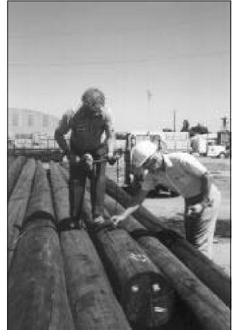
Core samples are examined to verify thorough preservative penetration in the ground-line zone.
