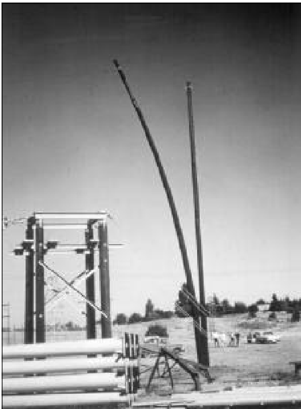
Full pole breaking tests were conducted on transmission poles; breakage occurred consistently well above ground-line.
